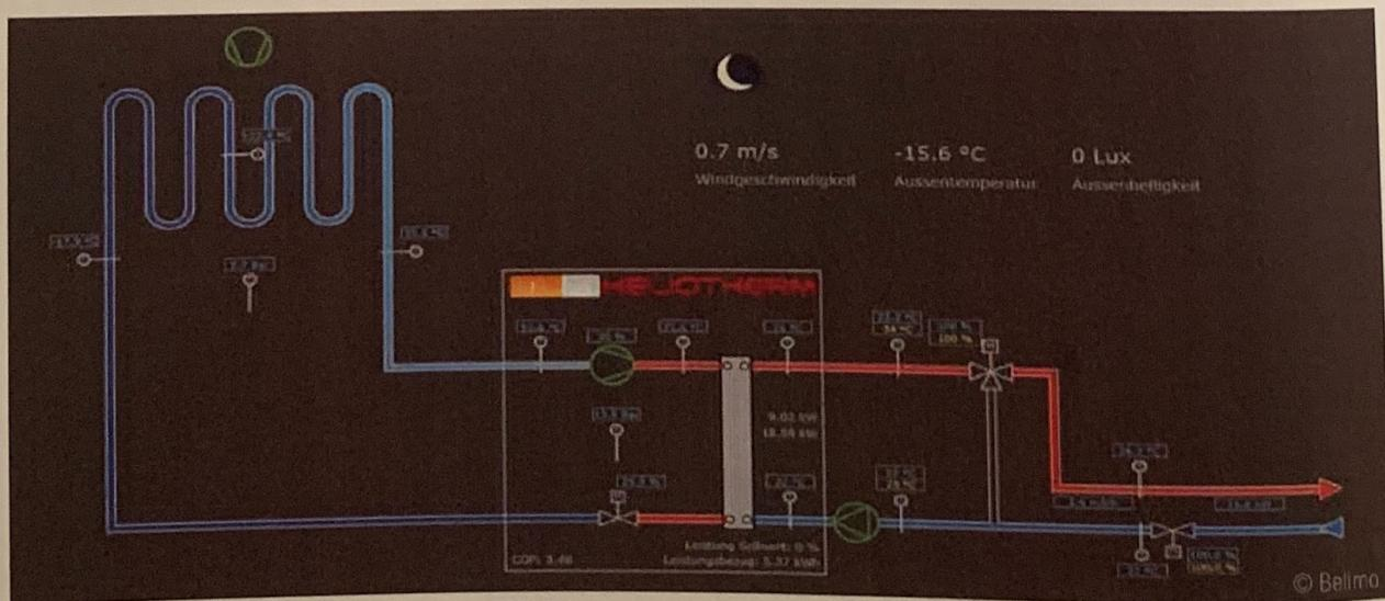
The picture shows the basic circuit diagram for the heat pump from the AZ systems AG management system.
